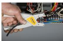
Jokari\_Sensor Special.jpg: With Sensor Special sensor cables can be stripped without damaging the inner conductors.
