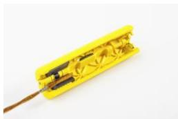
**Jokari\_Special 2:** By slightly snapping the sheathing the CAN-Strip will break it at the cut and strip it off with the internal rubber pads.
